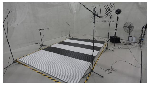
Figure 5.4 Measurement of sound absorption
