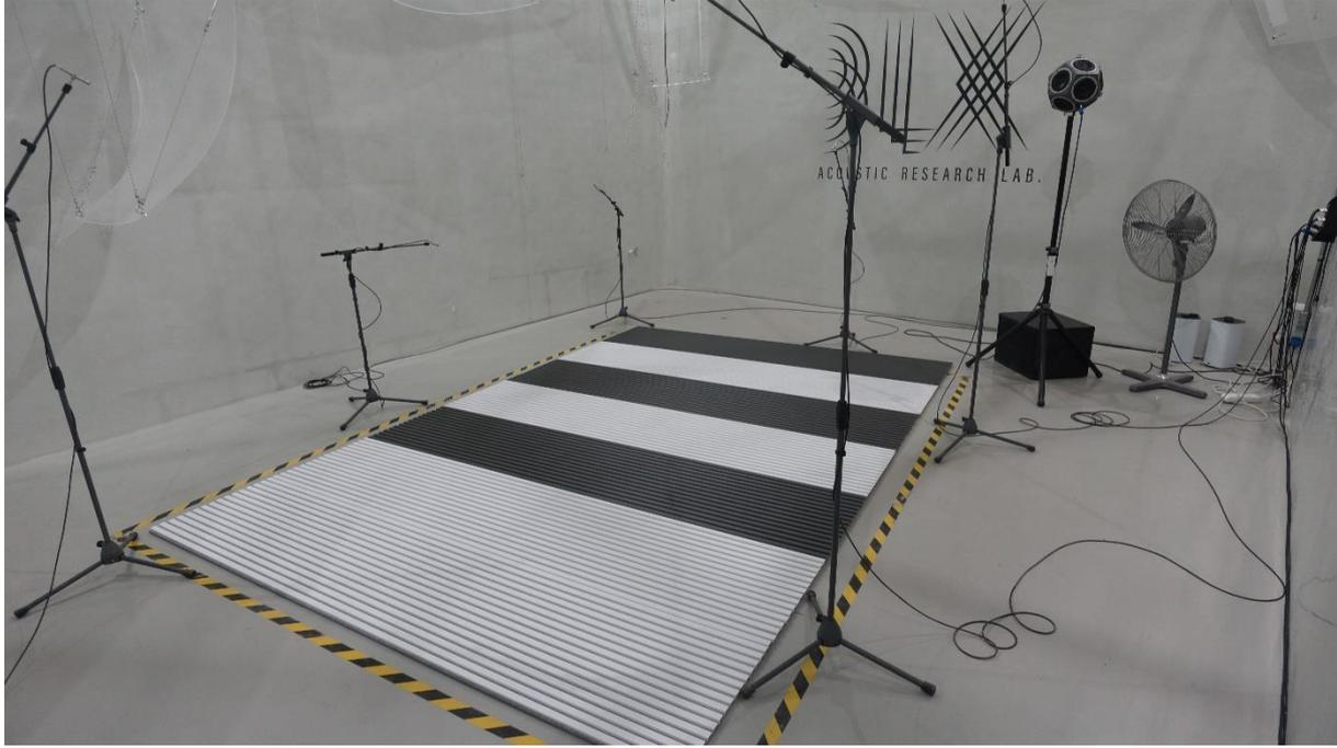
Figure 5.4 Measurement of sound absorption
